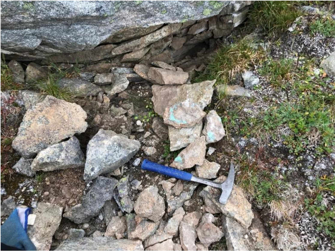
Figure 7. Monzonite dyke grab sample (72521) with Cu grades of up to 1.47% from the southwest area of Netalzul Mt.
