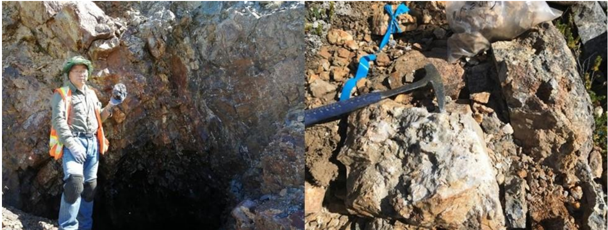
Figure 5. Adit 3 (left); one metre chip sample (#72013) from Adit 4 area with Ag grade @ 2915 g/t (right).
