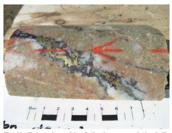
**Fig. 19.** Chalcopyrite- and bornite-bearing quartz vein in phyllic altered granodiorite at Carmax Mining's Eaglehead project. Photo by Bev Quist.
