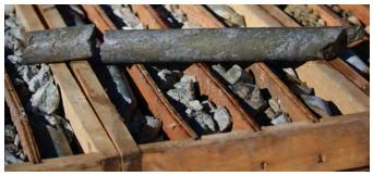
**Fig. 13.** Chalcopyrite-bearing drill core from Teuton Resources Del Norte project. Photo courtesy of Teuton Resources.
