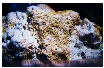
**Fig. 10.** Fine-grained electrum and pyrite in quartz-carbonate matrix from the Brucejack Cleopatra vein.
