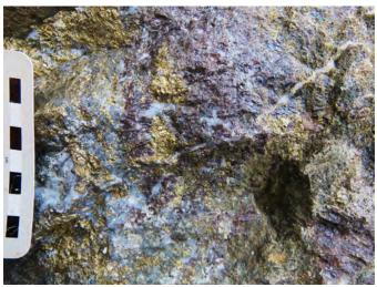
**Fig. 9.** Gold-bearing chalcopyrite and interstitial sphalerite from the Bob zone at Banks Island Gold's Yellow Giant gold project.
