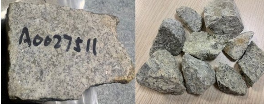
Figure 3. Monzonite outcrop (A0027511, Cu @ 0.27%) on left; and on right, monzonite drill core ( NET21-05, Cu @ 0.5%) from north area of Netalzul Mt project.
