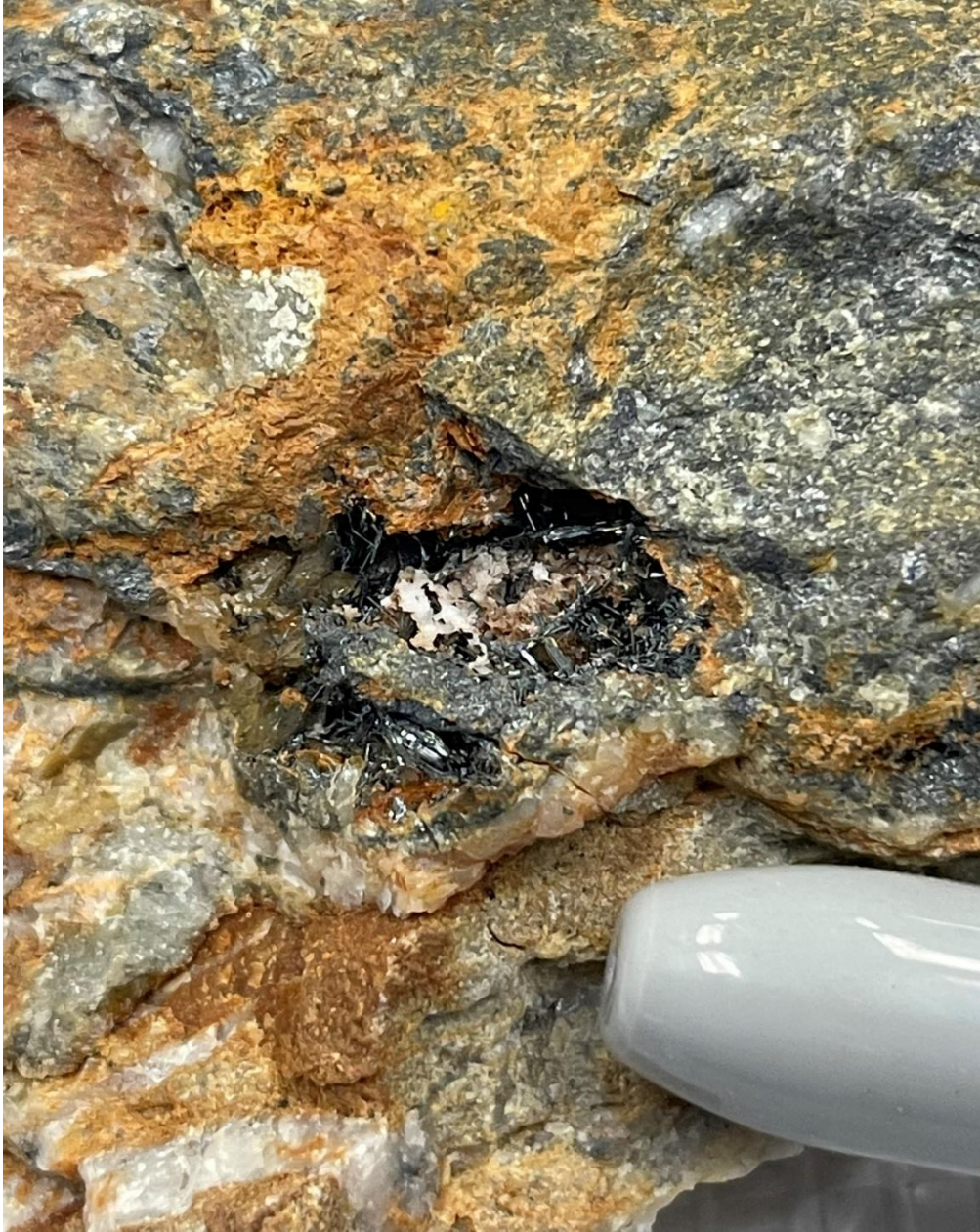
Figure 7. Antimony rock sample with typical striated prismatic stibnite crystals at KS zone 3.
