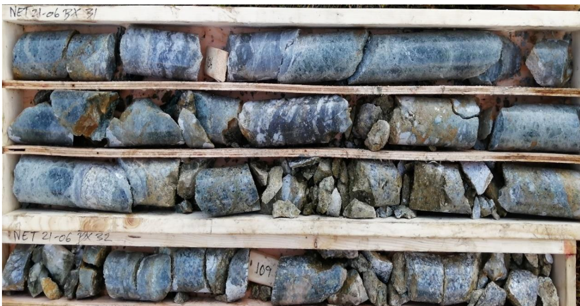
Figure 2. High-grade polymetallic mineral cemented quartz breccia core from 105.8 m to 109.3 m in hole NET21-05.
