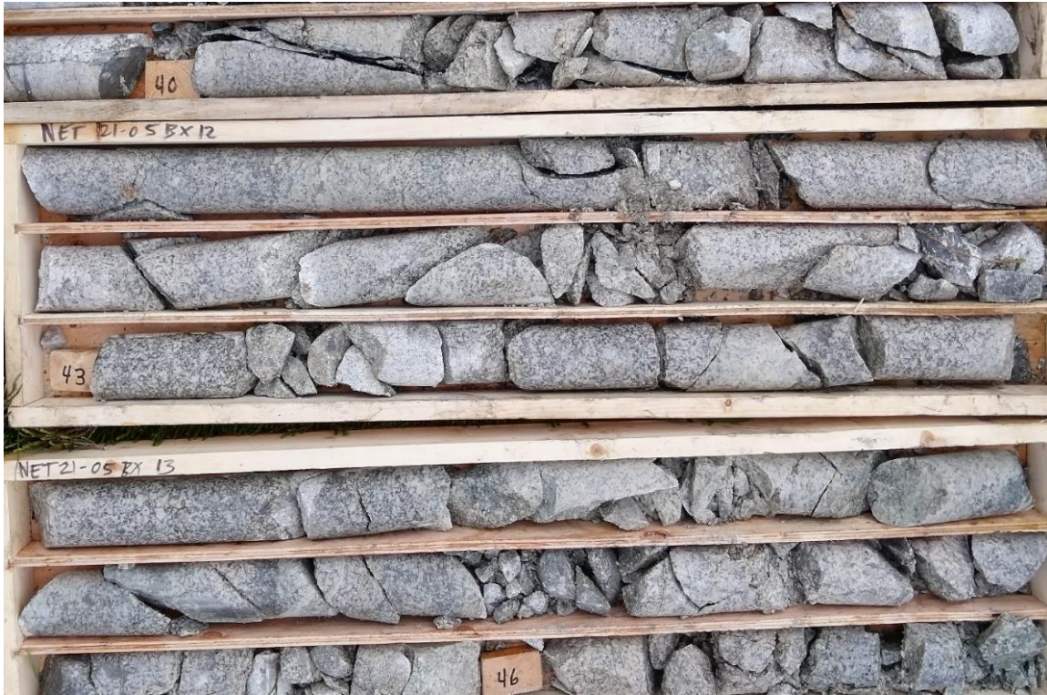
Figure 3. Core from 40 m to 46 m in NET21-05 showing mineralized monzonite porphyry dykes.
