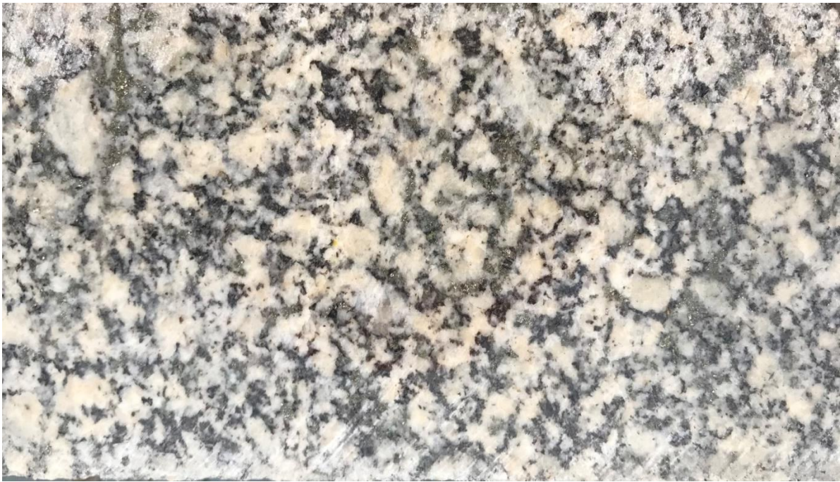
Figure 10. Core at 43.5 m from NET21-05 showing disseminated chalcopyrite and pyrite in monzonite.
