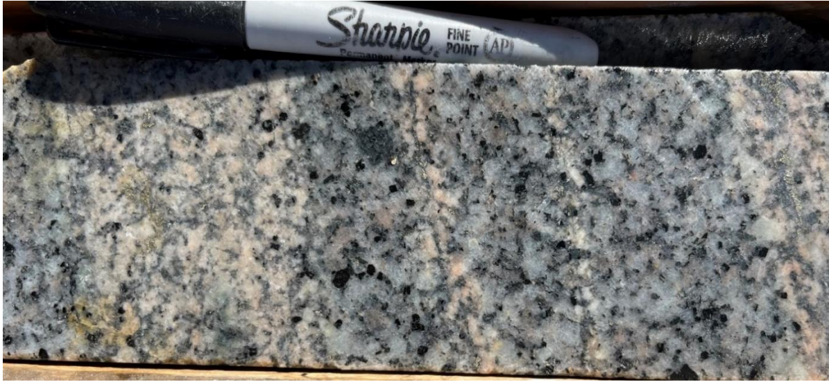
Figure 9. Core at 198 m in hole NET21-08 showing multiple altered K-feldspar and chalcopyrite-pyrite veins.
