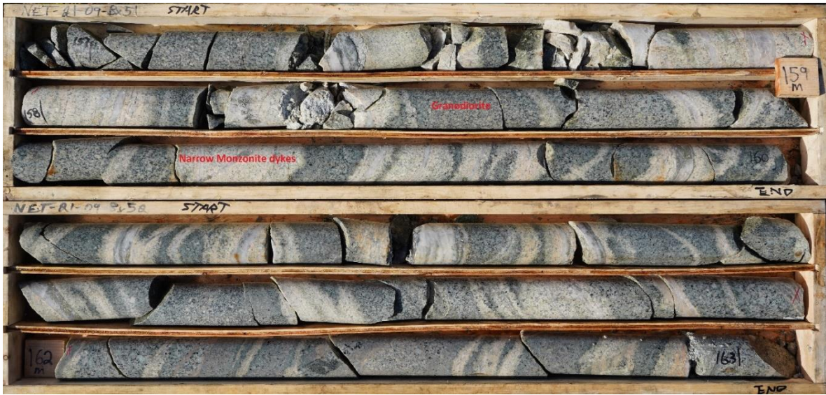
Figure 5. Core from 157 m to 163 m in hole NET21-09 showing multiple narrow monzonite dykes with Cu grades from 600 ppm to 900 ppm and Mo grades from 40 ppm to 600 ppm within granodiorite hosting rocks.
