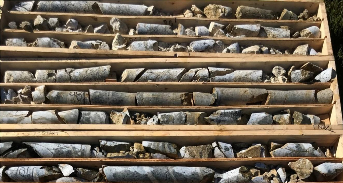
Figure 4. Core from 93.5 m to 100.5 m at NET21-06 showing multiple disseminated sulfide monzonite dykes; one large dyke from 98.0 m to 99.2 m with CuEq grade of 0.21% showing disseminated and vein sulfides and silicification.
