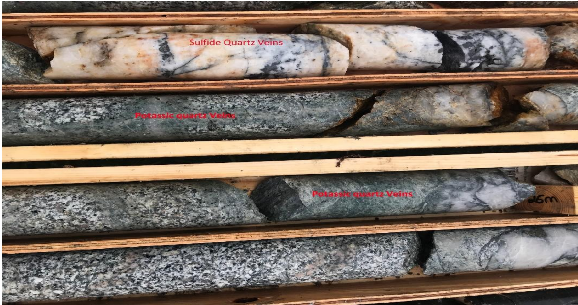
Figure 6. High-grade sulfide quartz veins with grades of 5.03% CuEq which include 0.57 g/t Au, 354 g/t Ag, 0.74% Cu, 0.42% Sb, 0.35% Pb and 0.44% Zn, and potassic altered veins (PQV) at hole NET21-01 from 23 m to 26 m.
