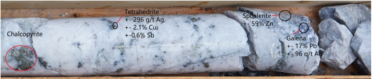
Figure 5. Core at 155.3 m to 155.6 m from NET21-02 shows high-grade Ag-Cu-Sb-Zn-Pb. Portable XRF analyzer reported Ag grades of up to 296 g/t, Cu grades of up to 2.1% from the tetrahedrite, 59% Zn from Fe-poor sphalerite and 17% Pb from mainly galena minerals.
