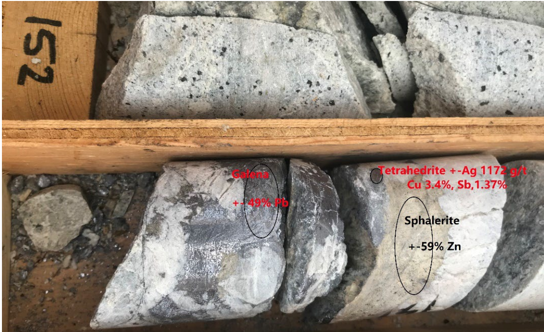
Figure 2. 10 cm thick massive galena-sphalerite-tetrahedrite-chalcopyrite vein at 151 m to 151.10 m from NET21-01. XRF testing shows high-grade Ag-Cu-Sb-Pb-Zn mineralization.
