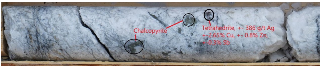
Figure 4. Core at 71.20-71.25 m from NET21-02 shows high-grade Ag-Cu-Sb. Portable XRF analyzer reported Ag grades of up to 386 g/t and Cu grades of up to 2.6% from the tetrahedrite and chalcopyrite mineral.
