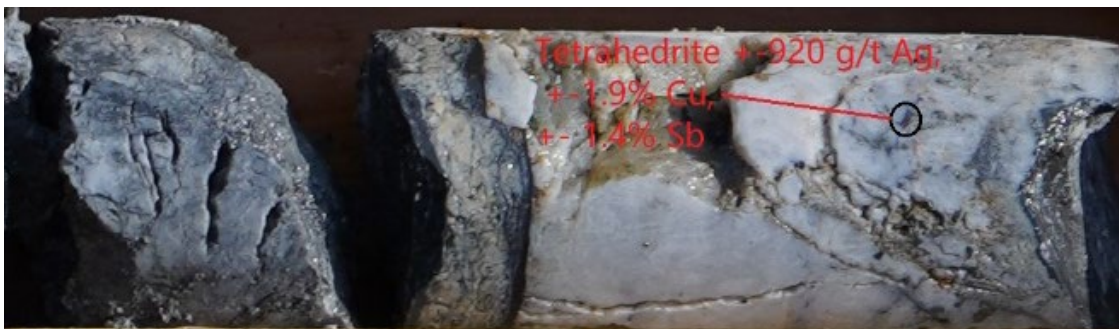
Figure 3. Core at 27.8 m from NET21-02 shows high-grade Ag-Cu-Sb. Portable XRF analyzer reported Ag grades of up to 920 g/t from the tetrahedrite mineral.
