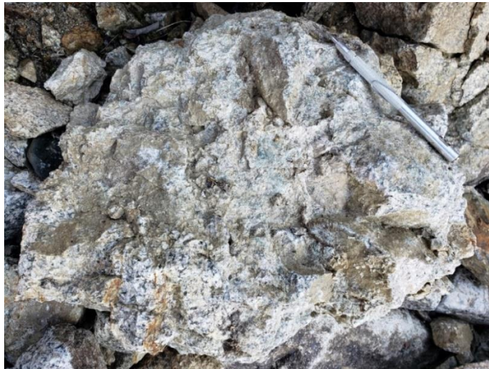
Figure 4: Outcrop of intrusive breccia sample A0027132 at Daisy, which is a clast of granodiorite set in the same composition of rock flour and smaller clasts; locally, hydrothermal quartz cements and malachite staining are visible; grab sample returned Cu of up to 0.10 %.
