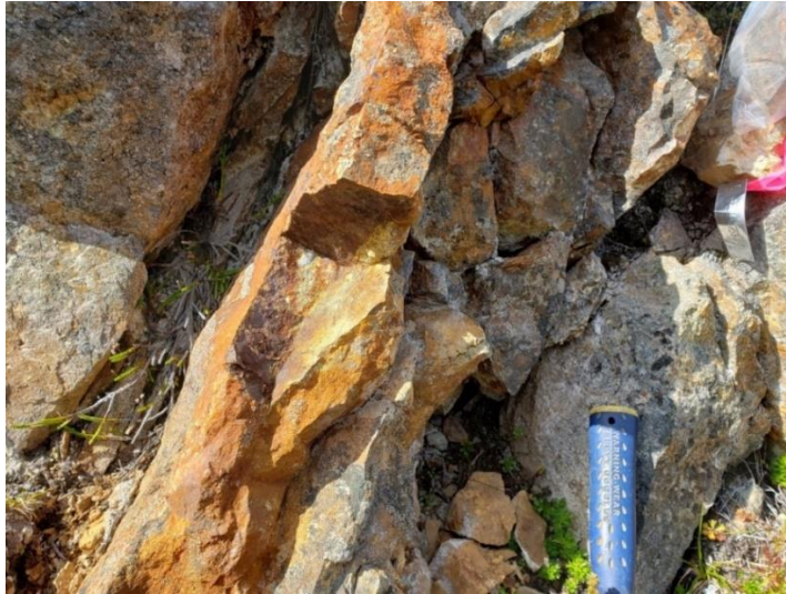
Figure 3: Outcrop of sample A0027126 quartz vein at Daisy, which returned Cu of up to 0.84 %, Au 0.114 g/t, Ag 47.1 g/t and 314 ppm Mo. The quartz vein structure zone could be one metre wide.
