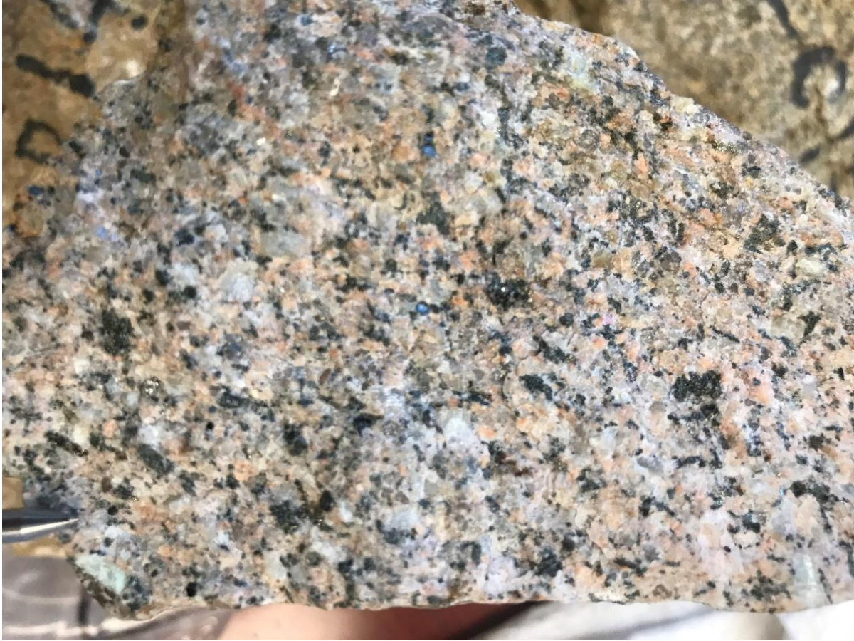
Figure 5, Altered Porphyritic Intrusion with Disseminated Pyrite and Chalcopyrite from Primary Ridge Porphyry Target
