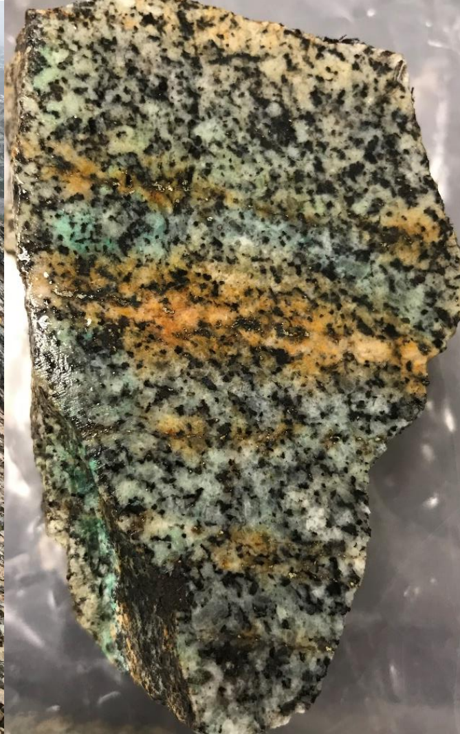
Chalcopyrite, potassium alteration veins & malachite alteration in biotite diorite
