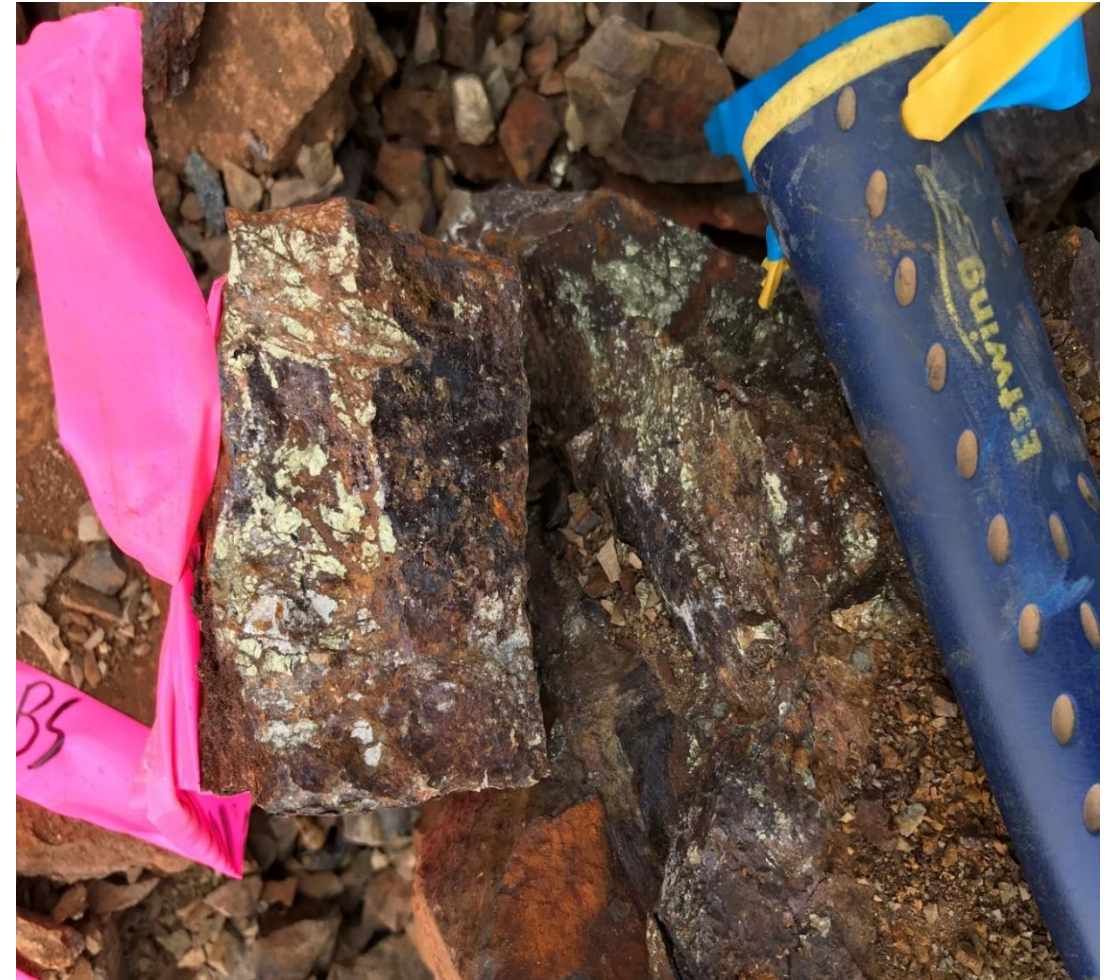
Massive sulphide (chalcopyrite) mineralization in tourmaline breccia zone (above)
